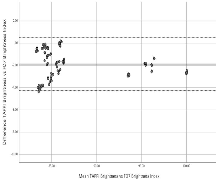
Figure 7. Konica Minolta FD-7 Tukey Mean-Difference Plot
