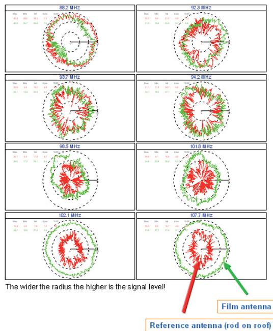
Fig. 11: Comparison of the FM-performance (88.2 – 107.7 MHz) between integrated film (green) and rod antenna (red)
