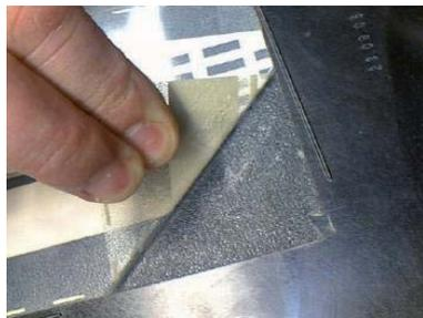
Fig. 10: Antenna film on polycarbonate body part after Kataplasma test
