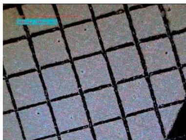
Fig. 9: Test sample after adhesion test
