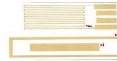
Fig. 7: Test layout for ink validation
