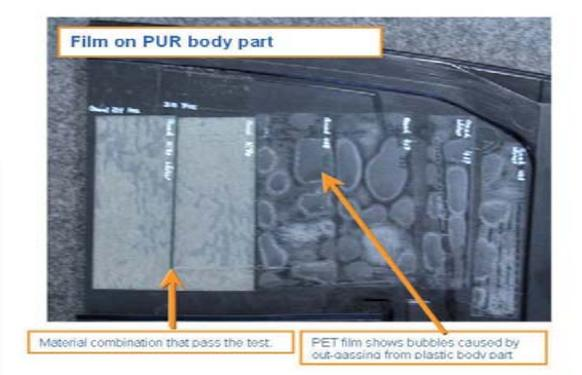
Fig. 8: Test samples after storing 4 days @ 85°C
