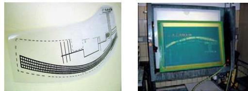
Fig. 5: Plotted film master and processing of screen printing form after contact exposure
