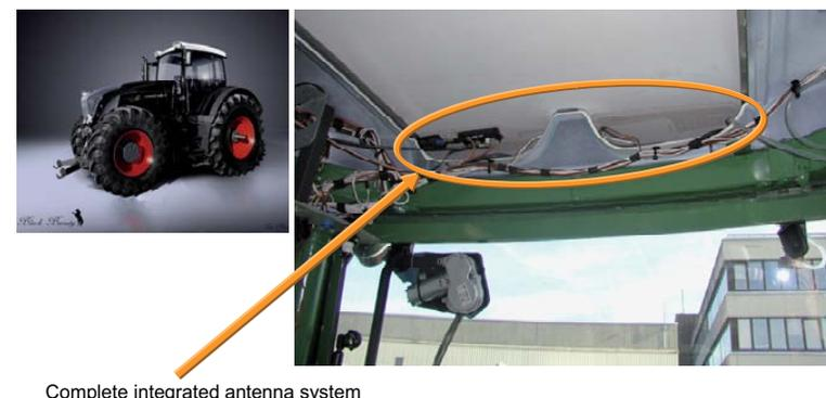
Fig. 12: First serial production of the developed integrated antenna system – AGCO Fendt X 900
