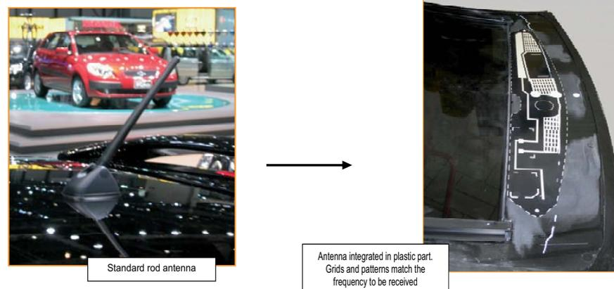
Fig. 1: Transition from rod to integrated antenna
