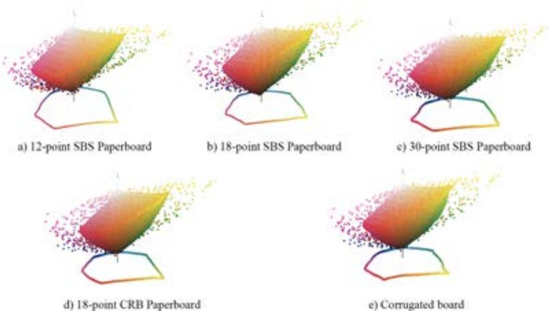
**Figure 3:** Colour Gamut of tested paperboards and corrugated board (With L\*a\*b\* values of spot colour original data for reference)
