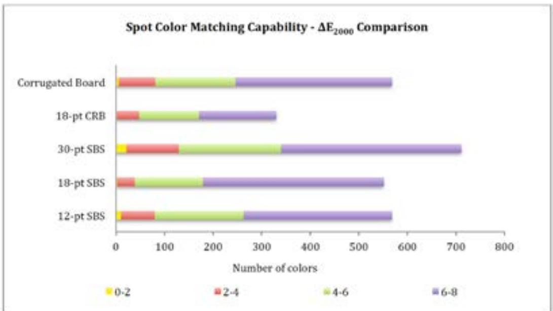
**Figure 4:** Spot colour matching capability for the teste paperboards and corrugated board
