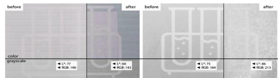
Figure 4: Photochromic (left) and hydrochromic (right) inkjet ink printed surface
