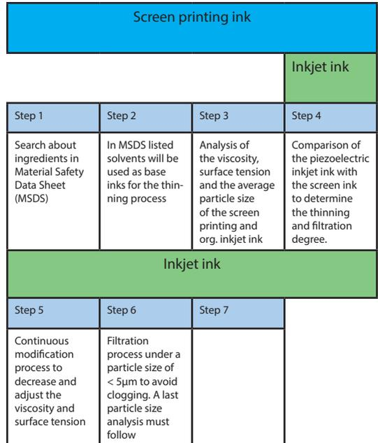
Figure 2: Modification process to develop a piezoelectric inkjet ink
