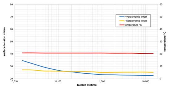
Figure 8: surface tension of developed inkjet inks
