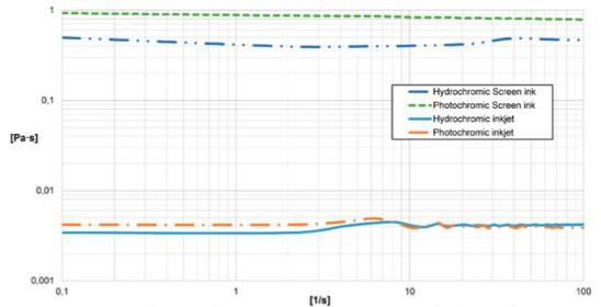
Figure 7: Flow behavior screen-printing and inkjet inks
