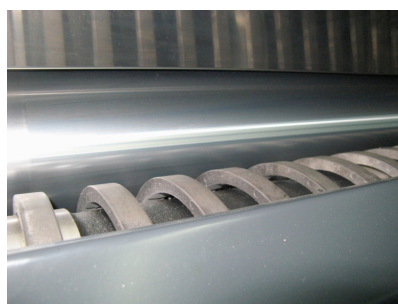
Figure 2. Photograph showing the ink deposition on the impression cylinder before printing.
