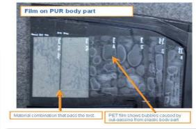
Fig. 8: Test samples after storing 4 days @ 85°C
