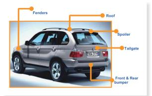
Fig. 2: possible antenna placements in a station wagon
