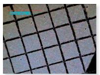
Fig. 9: Test sample after adhesion test
