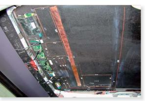
Fig. 4: Integrated antenna system realized with self-adhesive copper strips
