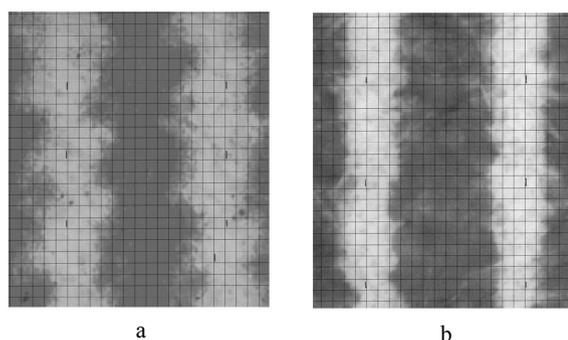
Figure 1: Microphotographs of test-charts areas with equally defined inked and non-inked widths of  $d = 2$  pixels or  $1/300$  of inch (200X: electrophotography a; ink jet b).
