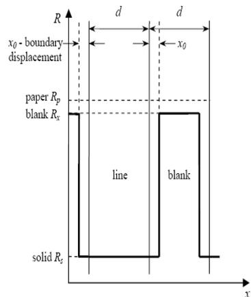
Figure 2: The distribution of reflectance across the elements after printing of the test-chart.
