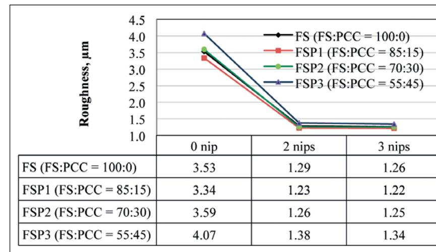
Figure 1: Parker Print-Surf Roughness measurement, μm
