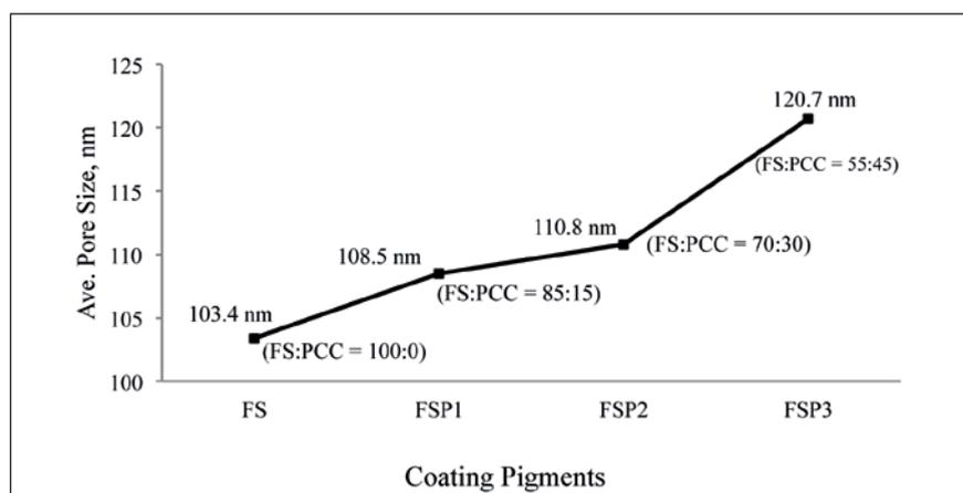
Figure 4: Average pore size measurement (calendered samples), nm
