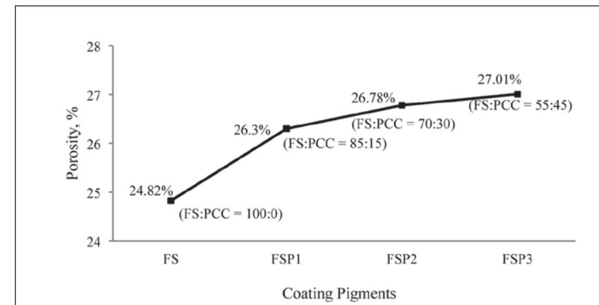
Figure 5: Porosity measurement (calendered samples), %
