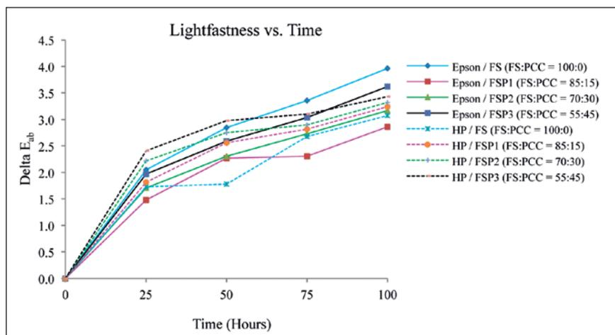
Figure 10: Color changes in coating formulations after light exposure for 100 hours
