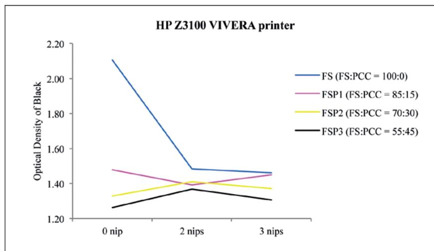
Figure 7: Optical density (black) comparison of each coating for the HP printer
