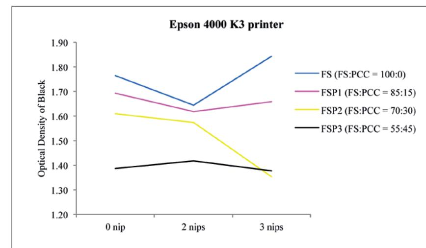
Figure 6: Optical density (black) comparison of each coating for the Epson printer
