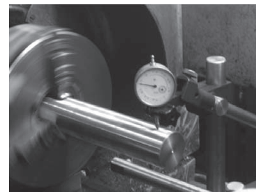
Figure 2: Vibration roll burnishing on a shaft
