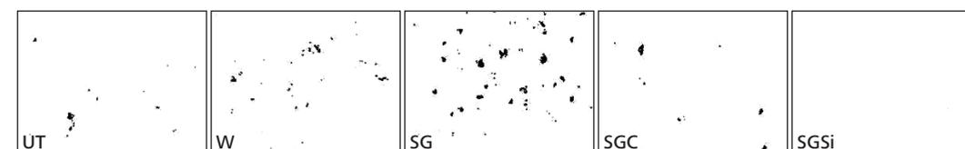
Figure 4: Representative picture of the reverse side of untreated and OX coated- and printed substrates. The black colour in the picture represents ink arising from front.
