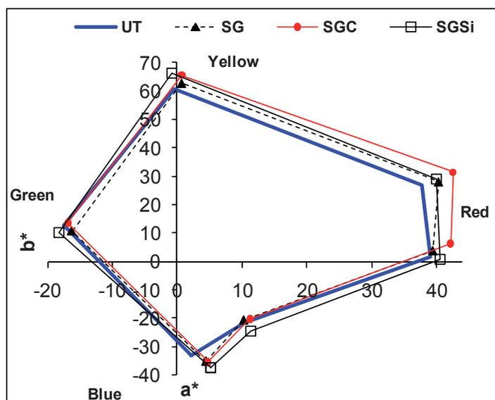
Figure 9: Colour gamut for untreated and OX coated substrates printed with inkjet. (Measured using Personal Image Analysis System PIAS-II from QEA.)
