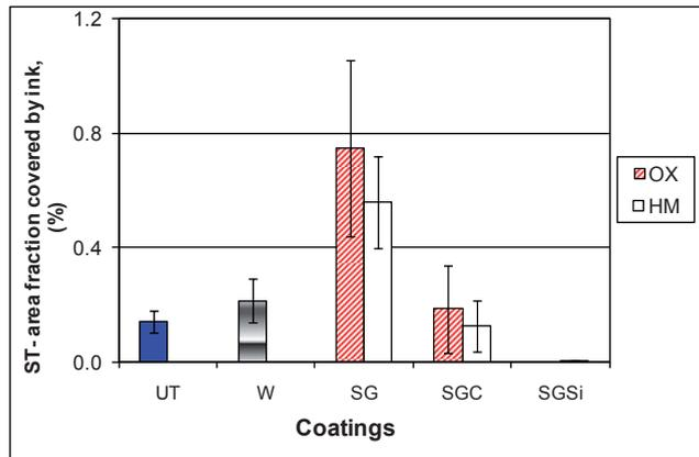
Figure 5: Strike-through expressed as a % area fraction of black ink present on reverse side of printed sample. Error bars indicate standard deviation.
