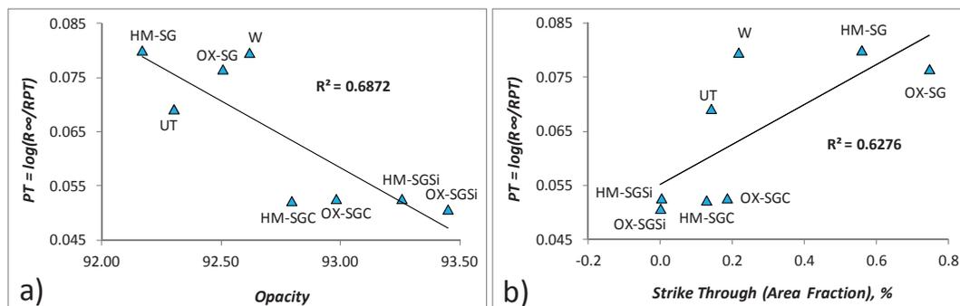
Figure 6: Correlation between: a) PT and opacity and b) PT and strike-through.
