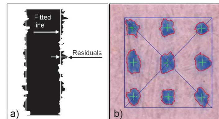
Figure 1: Schematic description of line raggedness (a) and method for evaluation of dot circularity (b).
