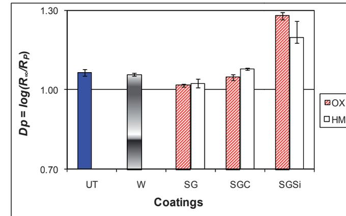
Figure 7: Print density (Dp) for substrates printed with black ink. Error bars indicate standard deviation.
