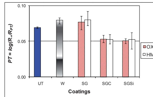
Figure 2: Print-through (PT) on the reverse side of the sample printed with pigment black ink. Error bars indicate range of value around the mean.
