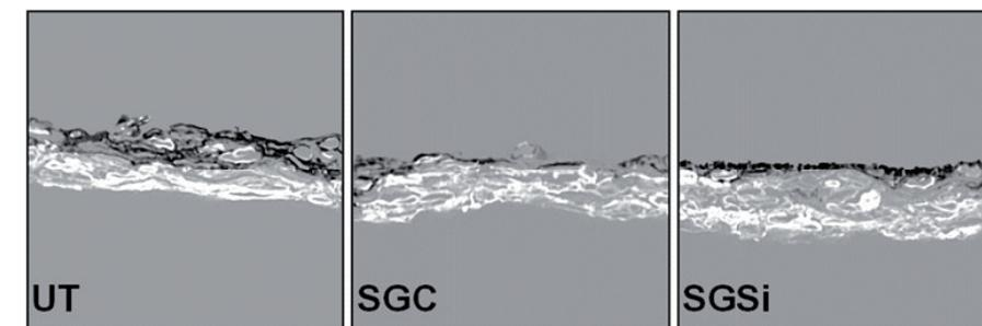
Figure 8: CLSM cross-sections of OX-coated newsprint printed with yellow ink. The black colour shows the ink distribution in x and z directions.
