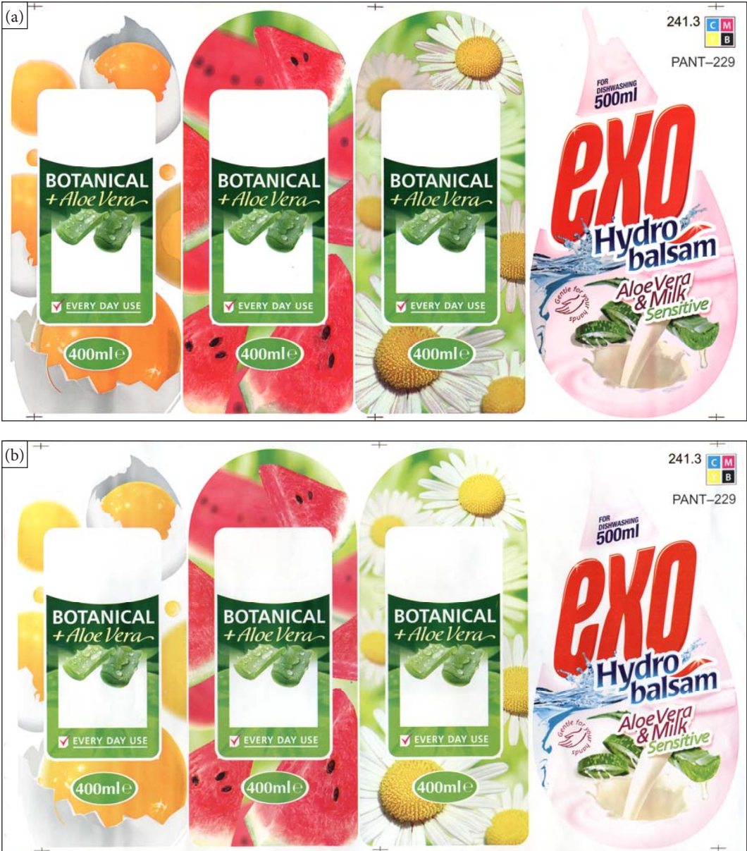
Figure 14: Comparison of tested print samples, a) Conventional screen, b) Using HD Flexo C46
