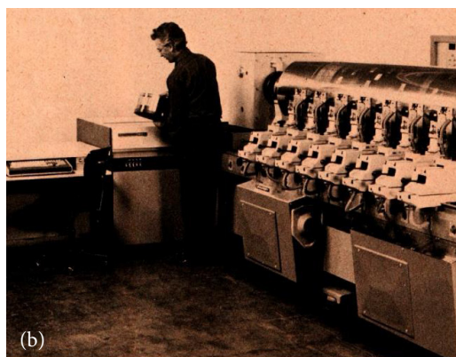
Figure 2: The special input unit for scanning the pasted-up negative reflection copies has had to be used to produce the signals for electronic engraving heads of HelioKlischograph (a). Such unit and copies preparation were omitted after introducing the first computerized color layout system HDP (b).
