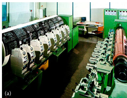
Figure 2: The special input unit for scanning the pasted-up negative reflection copies has had to be used to produce the signals for electronic engraving heads of HelioKlischograph (a). Such unit and copies preparation were omitted after introducing the first computerized color layout system HDP (b).
