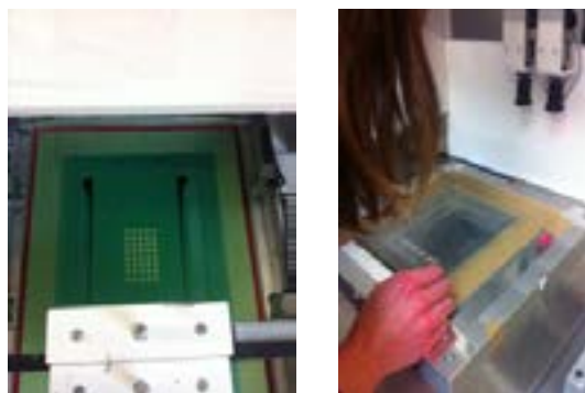
Figure 7: The pictures above show the silk screen form for the PEDOT:PSS rhombuses in the screen printing machine on the left, the silk screen form for the connectors consisting of silver paste on the right
