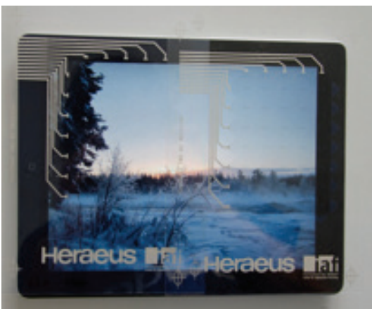
Figure 10: Finished transparent touchpad demonstrators of variants 6.1 and 6.2 in front of a tablet screen. As intended, the PEDOT:PSS rhombuses are hardly to see.
