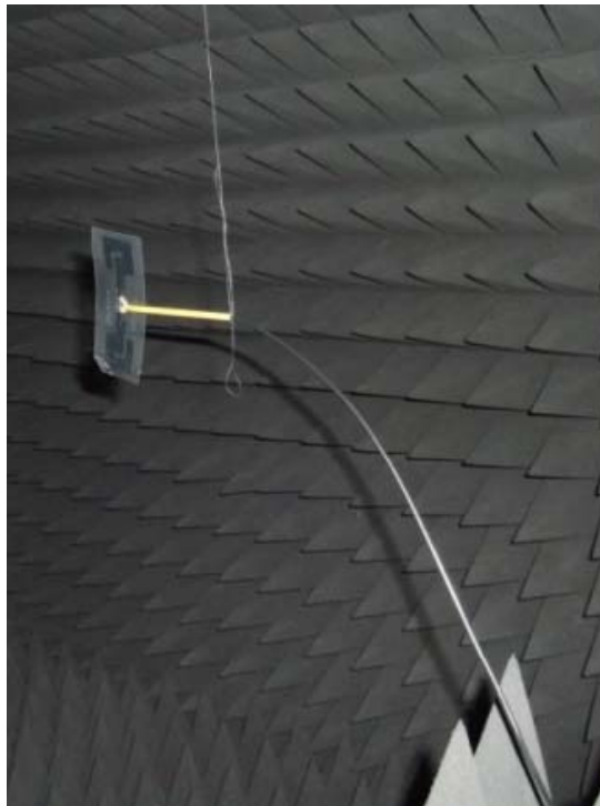
Antenna characterization in an anechoic chamber
