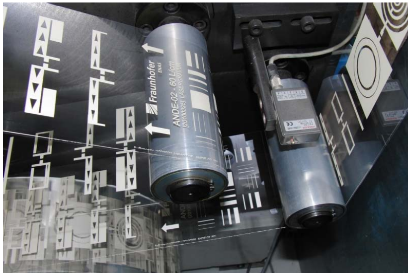
R2R gravure printed antennas on PET
