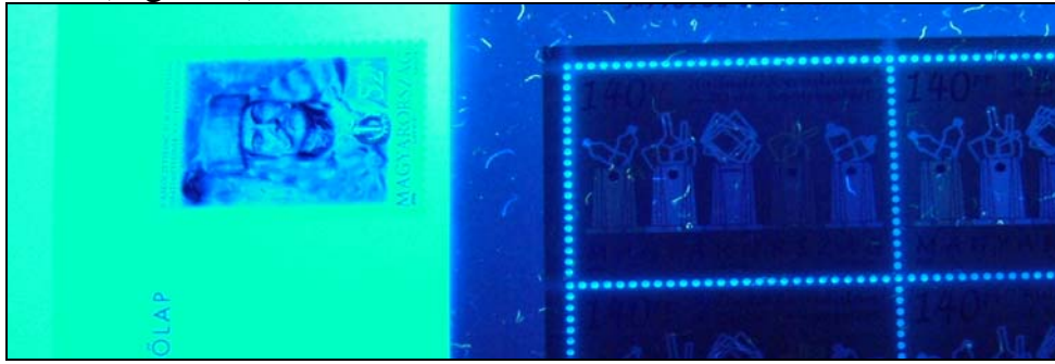
Figure 2. Proof (left) and postage stamps printed on special stamp paper (right) by UV-including radiation
