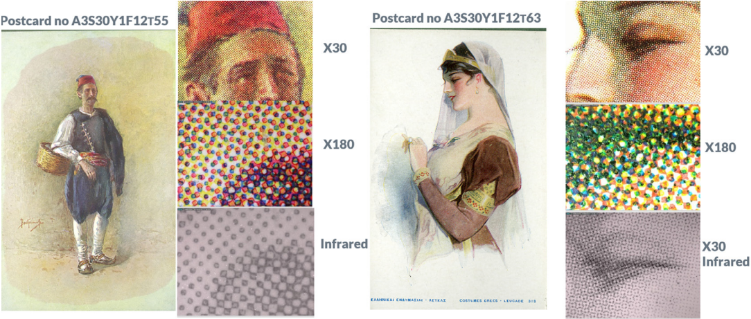
Figure 12: Examples of multispectral imaging for postcards with no A3S30Y1F12T55 and A3S30Y1F12T63 6
