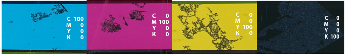
Fig.2. Assessment of the quality of prints using express-tests with TESA 4104 calibrated adhesive tape. Samples printed with Siegwark inks (CMYK on a white colour)
