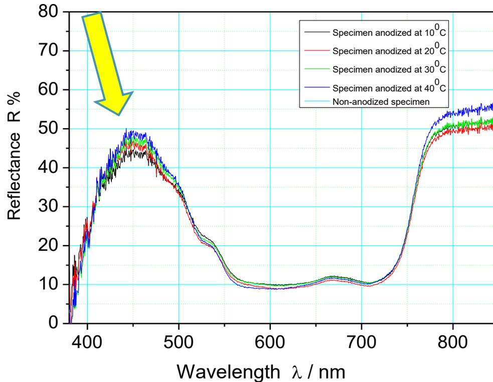
▶ **Fig. 1.** Reflectance spectra (R%) of digital printed specimens of anodized aluminium in P.A. in the range of 380-730 nm
