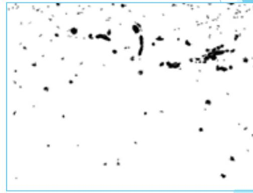
In all cases 2.6-3.6% of printed area was covered by aggregates only 2.3% on specimen anodized at 30°C
