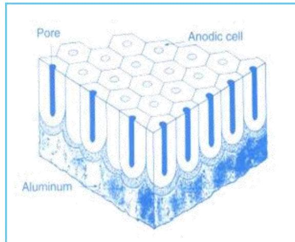
▶ These coatings are thick (5-35  $\mu\text{m}$ ) and if sealed subsequent to anodizing, give very good corrosion resistance as well as being harder and more wear resistant.
