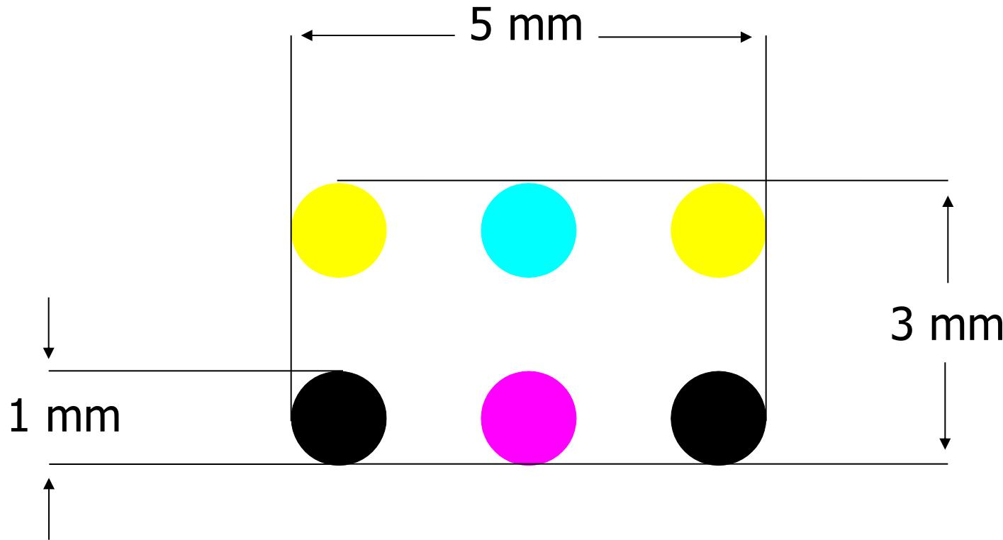
Techkon register mark → Techkon 920 Register control unit
