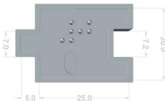
Figure 1. The CAD plate model with the Braille and Latin numbers.
